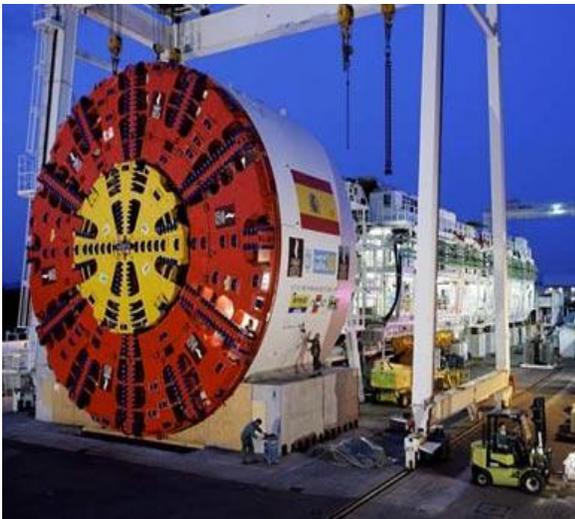
This is a tunnel boring machine that must work uninterrupted. These types of machines are only stopped for maintenance and if the machine was to shut down for any unscheduled reason, it takes 5-7 hours to restart. Adding the CPS feature was mission critical.
